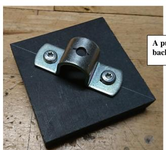
A pull handle is mounted on the backside of one of the MDF plates.
